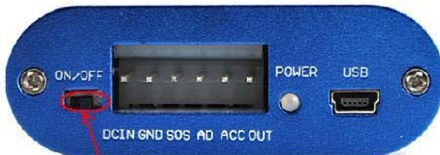
Push the button from OFF to ON side to turn on tracker
